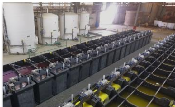
Solvent extraction ("SX") circuit at the White Mesa Mill producing high-purity NdPr
