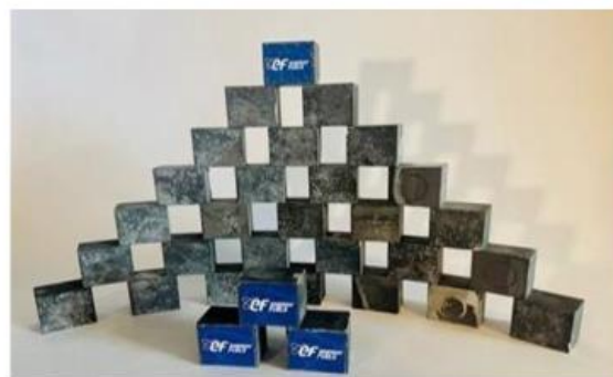
Production of NdFeB alloy sintered blocks from Energy Fuels' NdPr oxide
